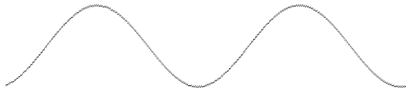
Figure 10. Demodulated signal after low pass filter
